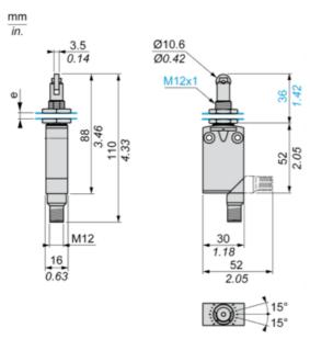
e : 8 mm max, panel cut-out Ø 12.5 mm, fixing nut thickness 3.5 mm.
